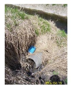
April/May of 2006 a straight pipe septic system was monitored for e.coli bacteria. Stream/pipe monitoring continued after a mound system was installed in May 2006.
