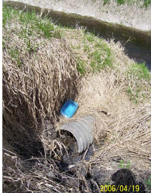
Sampling drainage tile outlet near drainage ditch.
