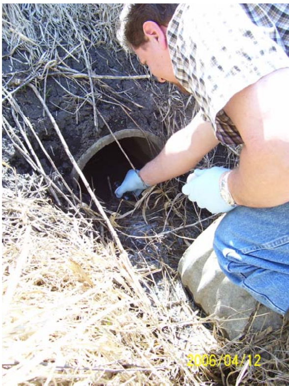
Sampling drainage tile outlet near drainage ditch.
