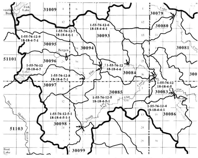
Figure 15. Hydrologic relationships of minor watersheds using CSAW numbering system.
