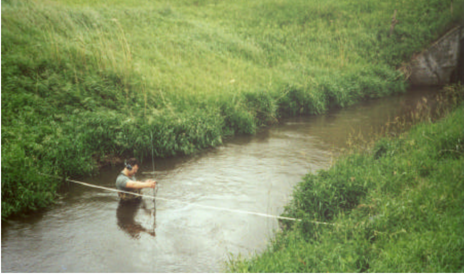
Photo 10. Stream flows taken for stage-discharge rating curve development during higher flows at site 1 on CD 13.
