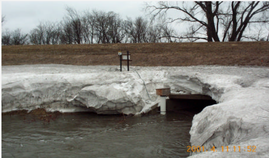
Photo 4. April 11, 2001. Spring runoff conditions at site 2. The monitoring sites had to be dug into the snow pack in order to capture the spring runoff conditions.
