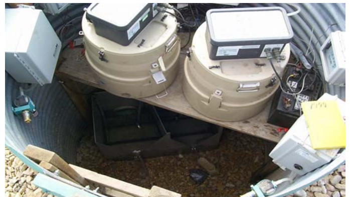
Figure 3. ISCO samplers collect tile water samples. A pair of weirs, in tandem with “pressure bubblers”, is used to measure the flow rate from Field 1 and Field 2.
