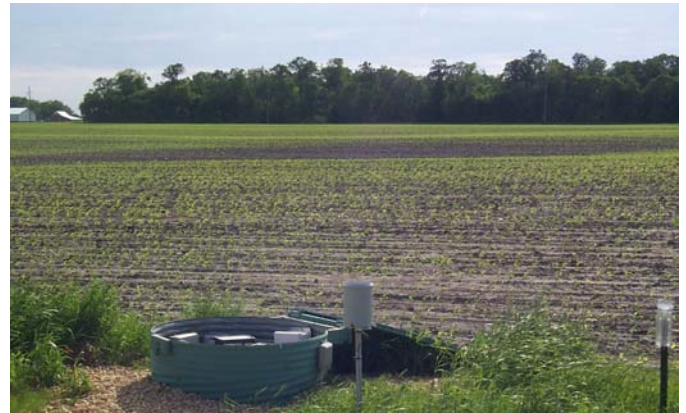
Figure 3. ISCO samplers collect tile water samples. A pair of weirs, in tandem with “pressure bubblers”, is used to measure the flow rate from Field 1 and Field 2.
